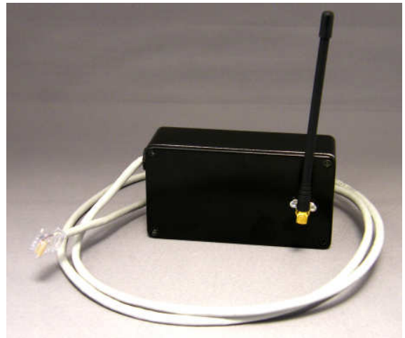
Main control unit RF antenna
